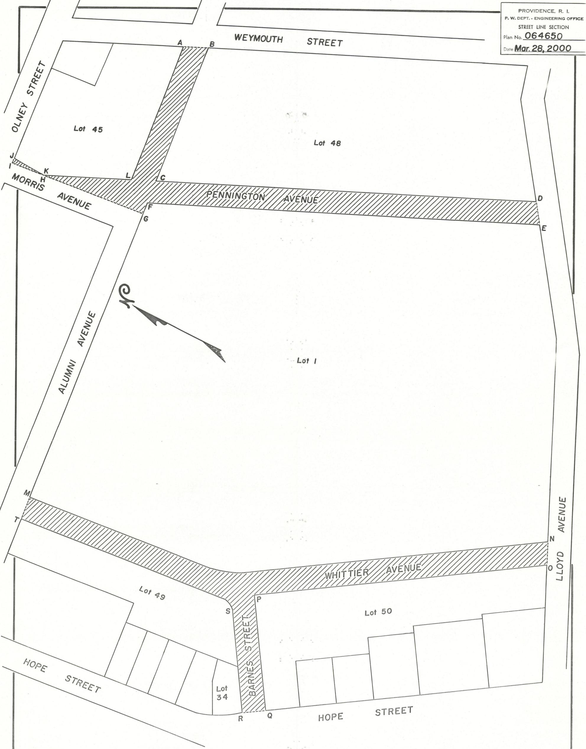
NOTES: Cross-hatched areas (A-B-C-D-E-F-G-H-I-J-K-L-A) & (M-N-O-P-Q-R-S-T-M) indicate proposed abandonments. No sewer easement required.
