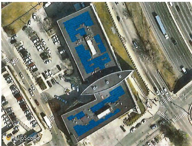
Public Safety Complex solar array blueprint
