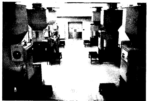
Introduction of chemicals into the treatment process is automatically controlled by modern chemical feeding machinery.
