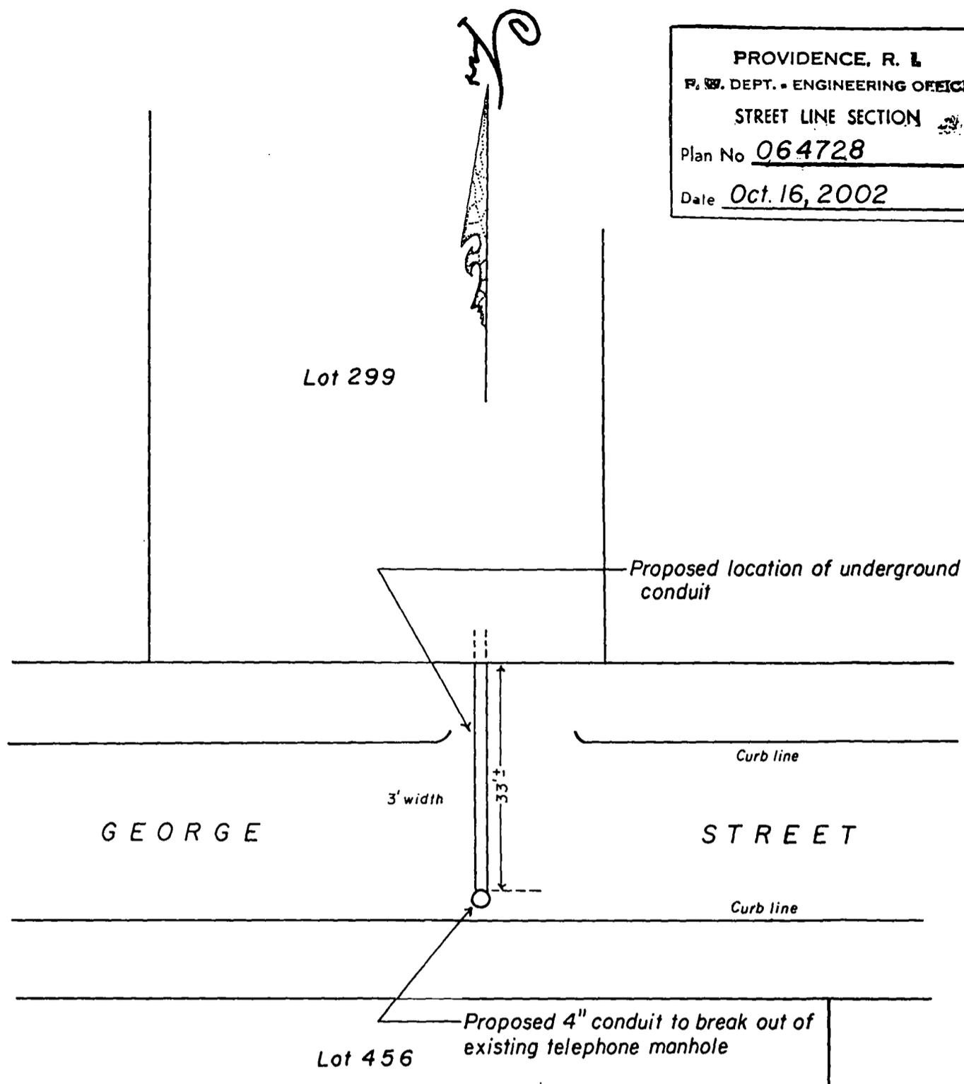
NOTES: Plan showing proposed easement for underground conduit for Cox Communications.
