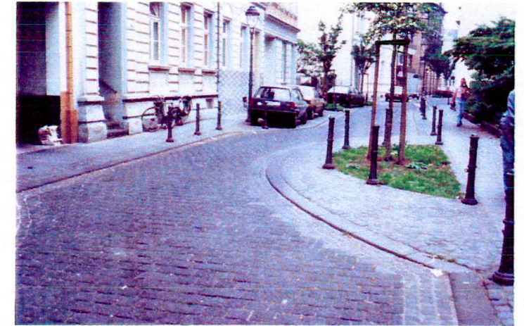
56. An elegant carriageway constriction incorporating tree, bollards and paving. Bonn, Germany. (Photo: Paul Murrain)
