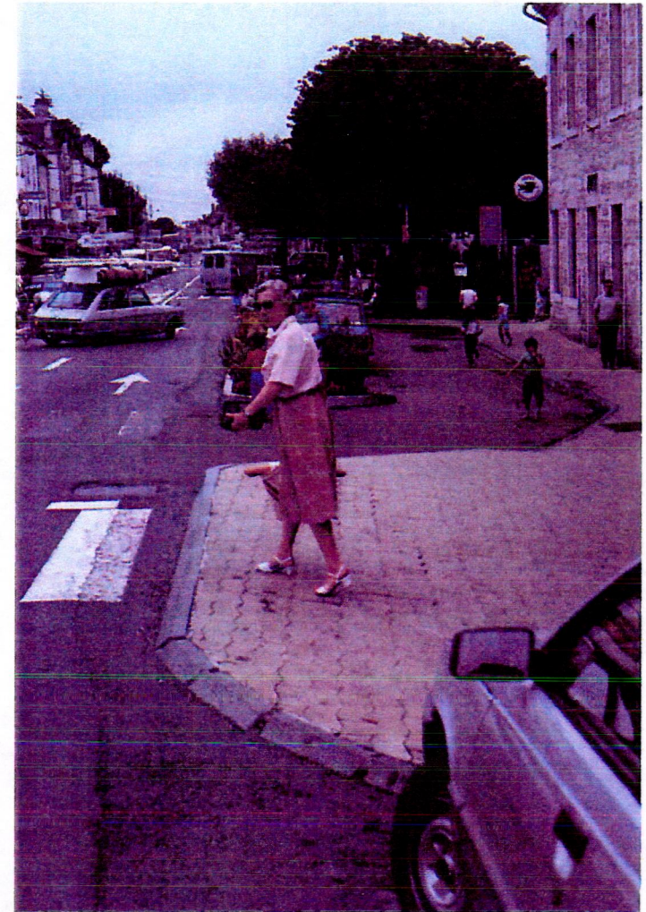
39. Sidewalk extensions improve visibility and shorten the crossing distance as well as narrowing the travel lane. Souillac, France. (Source: Devon County Council, 1991)
