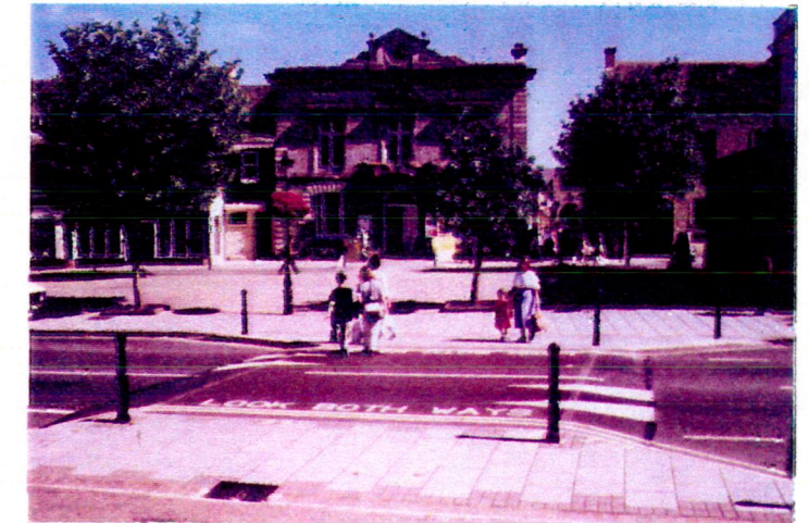
41. Speed table combined with sidewalk extension and crosswalk illustrating the principle for the Asa Messer precinct. Witney, England (Photo: Paul Murrain)
