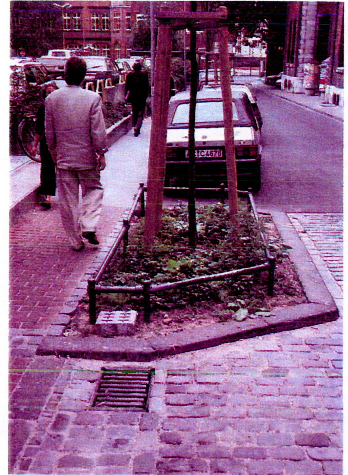
33. Tree given good protection and support using elegant materials. Aachen, Germany (Source: Devon County Council, 1991)
