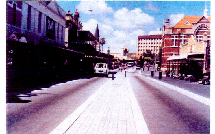
63. Here the median uses bollards and textured paving. Both are possible between trees. Fremantle, Australia. (Photo: Paul Murrain)
