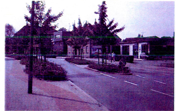
49. A central island reducing carriageway width and assisting in the creation of a gateway. Herne, Germany. (Photo: Tim Pharoah)
