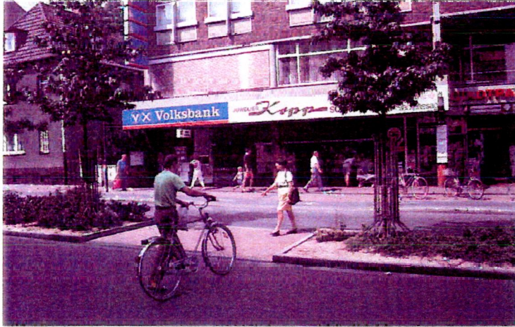
61. Medians giving pedestrians a refuge between the two travel lanes. Langenfeld, Germany. (Photo: Tim Pharoah)
