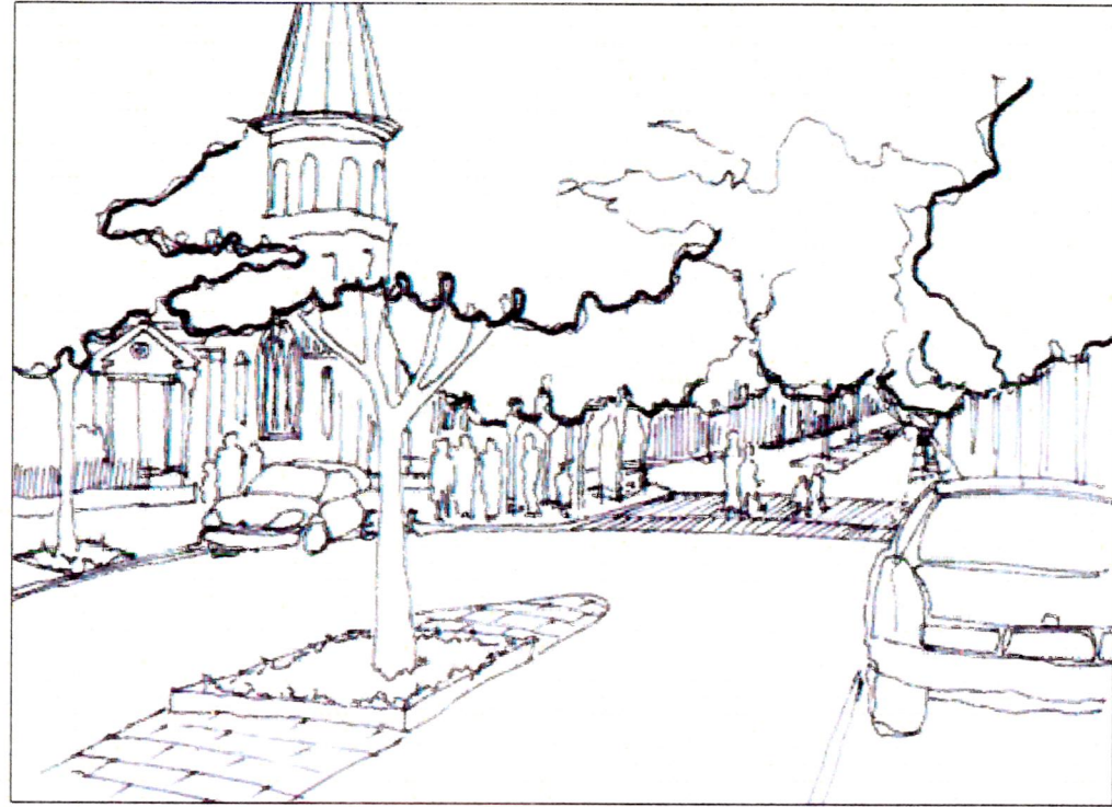
82. Hmong Church sketch proposal showing median, sidewalk extension and speed table in place. (Drawn by: Virginia Branch)
