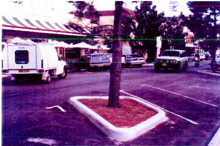
52. A tree planted further out into the street. In this case, it is to define angled parking. But it has a significant narrowing effect on the travel lane. Freemantle, Australia. (Photo: Paul Murrain)
