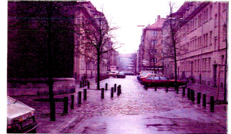
84. Paving, bollards and tree mark out a lateral shift. Nuremberg, Germany. (Photo: Tim Pharoah)
